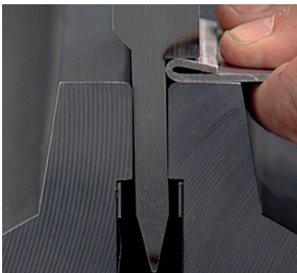
Pre-bend and flattening in the same tool.
